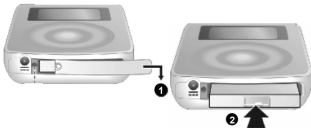
1. Push the battery cover to the side, so that the battery compartment is visible.
