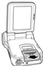
2. Insert the SD/SDHC card into the card slot, as illustrated.
